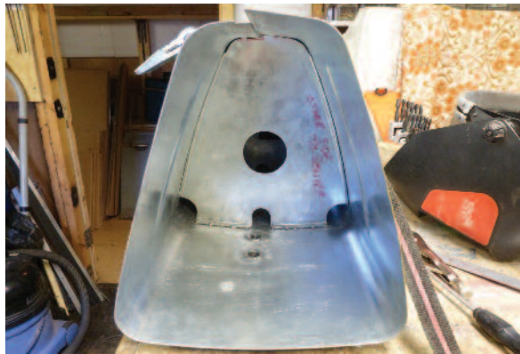
Picture 36. Second baffle welded into place.
