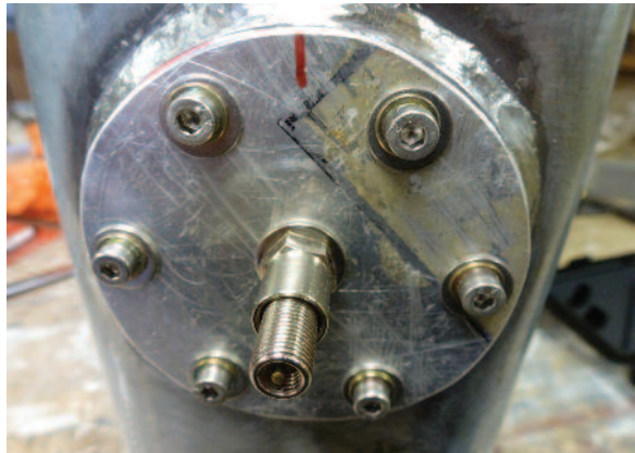
Picture 42. Tank sender plate with valve to allow a foot pump to be attached
