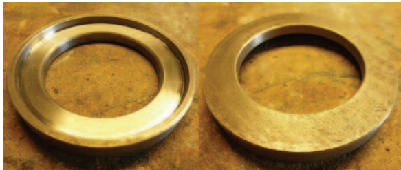
Picture 31. Top and bottom of the sender unit plate prior to drilling the sender securing holes.
