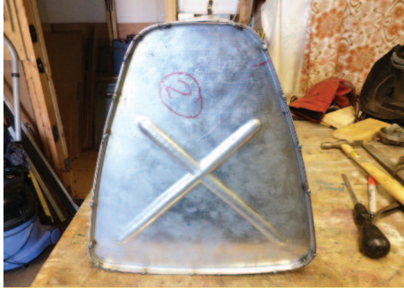
Picture 33. End plate tacked into place.
