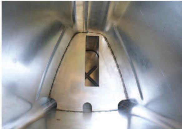
Picture 34. First baffle welded into place.
