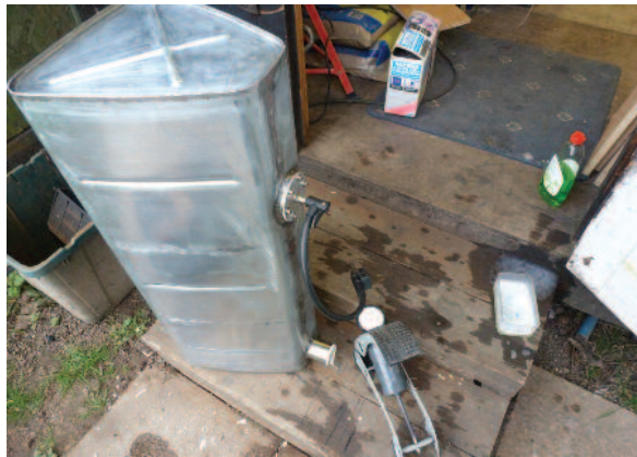
Picture 43. Pressure testing the tank..
