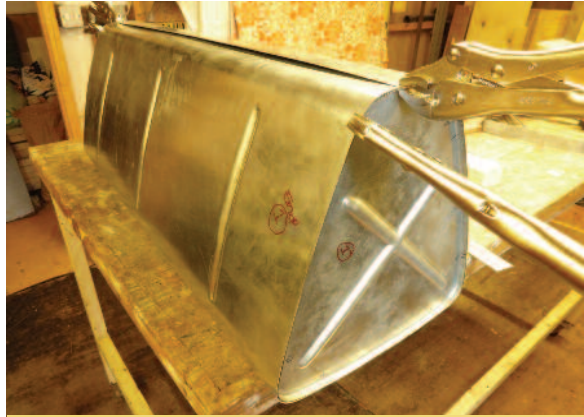
Picture 27. Trial fit of the end plates.
