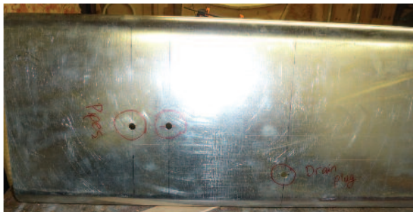
Picture 32. Bottom of the tank showing the holes for the two fuel pipes and the drain
