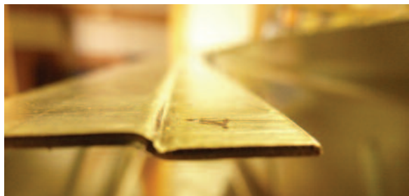
Picture 29. The shape of the metal after the joggler has been used.
