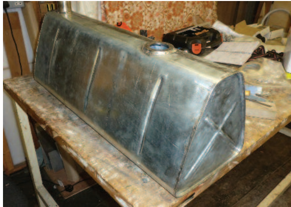
Picture 39. Fully welded tank
