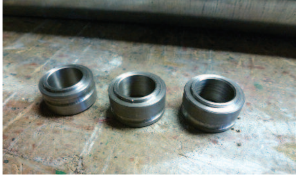
Picture 30. The three bosses fitted to the bottom of the tank.
