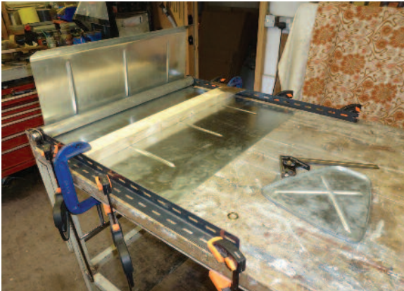
Picture 24. Second bend showing the piece of wood used to clamp the sheet.
